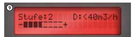
The Optiflow NT multi-function display indicates a colour-coded rendering of the drying installation's efficiency.
