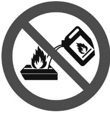
Do not fill fuel into the open flame
