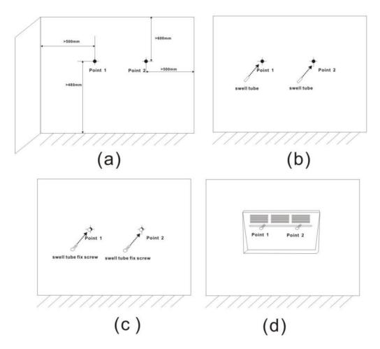
\* If there has ceiling or any articles on top of unit, the distance should be bigger than 600mm. The small distance will cause distortion and fire.
