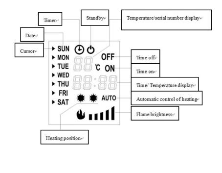
**Temperature and serial number display:** Normally it displays the room temperature; while setting the temperature, the setting temperature is displayed; When setting the timer, serial number is displayed.
